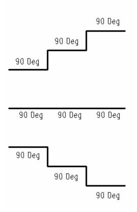
The same can be said for directional surveying. It is highly erroneous to assume a constant curve (as with the Minimum Curvature method), when the actual well path is
